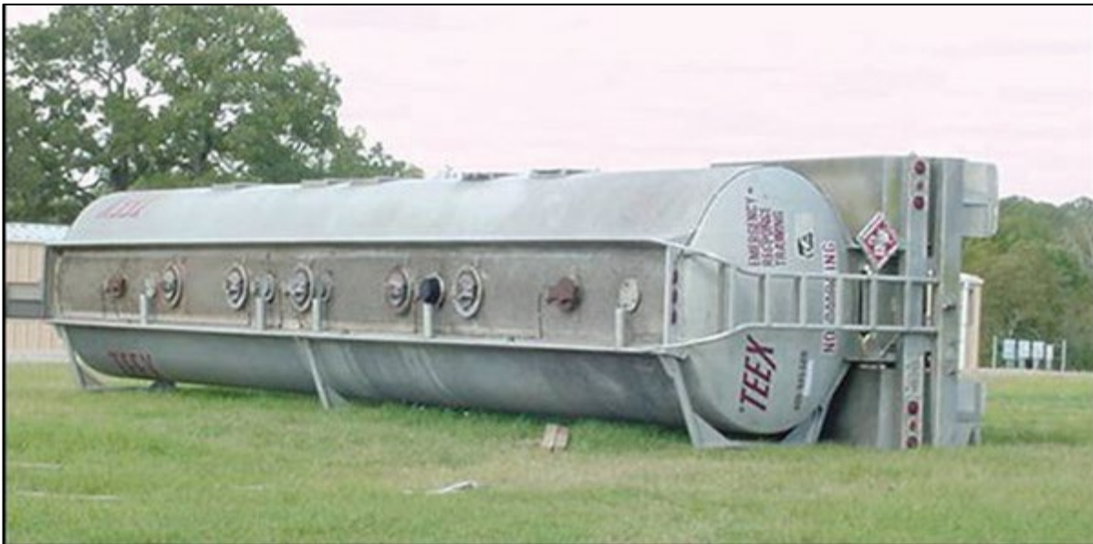
Figure 4.5: Overtuned MC-306/ DOT-406 Cargo Tank
