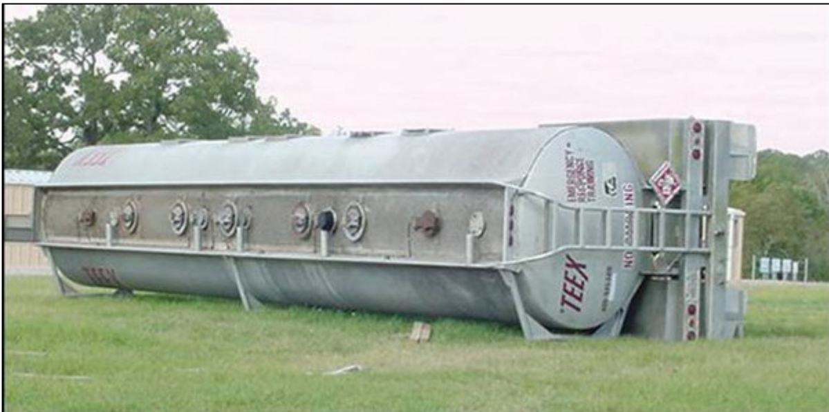
Figure 4.5: Overturned MC-306/ DOT-406 Cargo Tank
