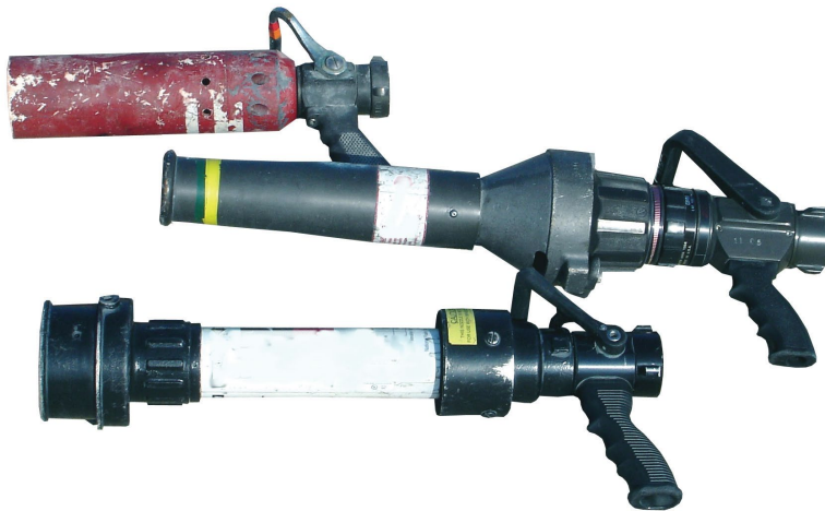
Figure 6.6: Air Aspirating Nozzles
